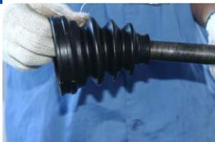
Remove the defective boot from drive shaft
