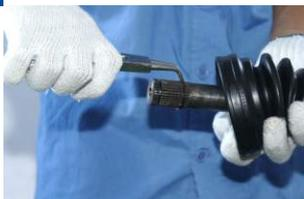
Place circlip in the groove of ball hub
