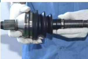
Check closely the fit of retaining clip. Caution! Boot rim must be in full contact with joint
