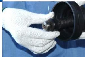
Joints outfitted with disc spring and thrust washer these have to be installed in their correct position on the shaft
