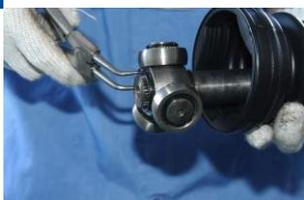
Place circlip in groove of ball hub, shanks of circlip lie in the outer recess
