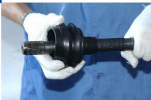
Place boot in the correct position between ridges of shaft
