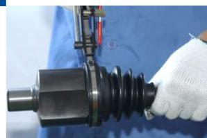
Lock retaining clip with pliers
