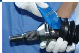
Fill remaining grease into the boot
