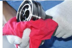
Remove waste grease and clean the joint
