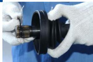
If the circlip has to be positioned inside, place it in the groove of the shaft
