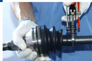
Lock retaining clip with pliers
