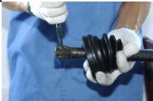
Pull off boot from circlip
