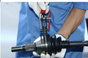
Lock retaining clip with pliers
