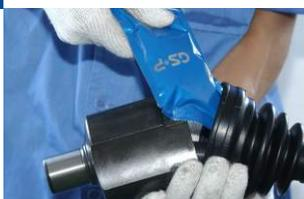
Fill remaining grease into the boot
