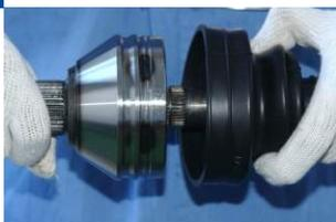
Plug joint on shaft until splines of shaft and ball hub are in line
