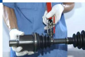
Lock retaining clip with pliers
