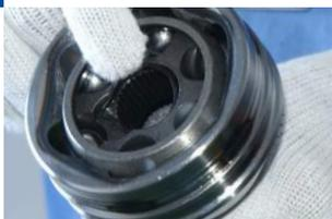
Place circlip in the groove of ball hub, the shanks of circlip lie in the outer recess
