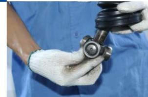
Using a plastic or rubber hammer, knock joint from shaft
