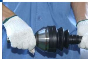
Pull boot on joint into correct position
