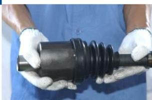
Apply retaining clip by hand as tightly as possible
