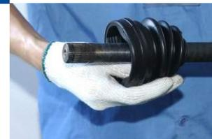
Place boot in correct position between ridges of shaft
