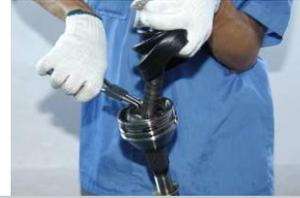
Expand circlip and pull joint from shaft by tapping with a plastic hammer on the joint's face
