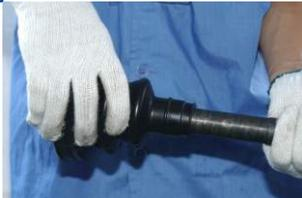
Remove the defective boot from drive shaft
