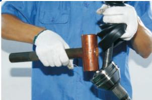
Joints outfitted with inside-positioned circlip (invisible) have to be pulled off the tapping with a plastic hammer on the joint's face
