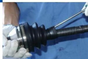
Remove the air from inside by lifting the end of the casing with a lever
