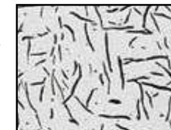
Graphite flakes in the microstructure of the XG-150 cast iron
